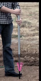
To install, insert the tip of the slide-driver (sold separately) into the cavity of the Stake All™.
